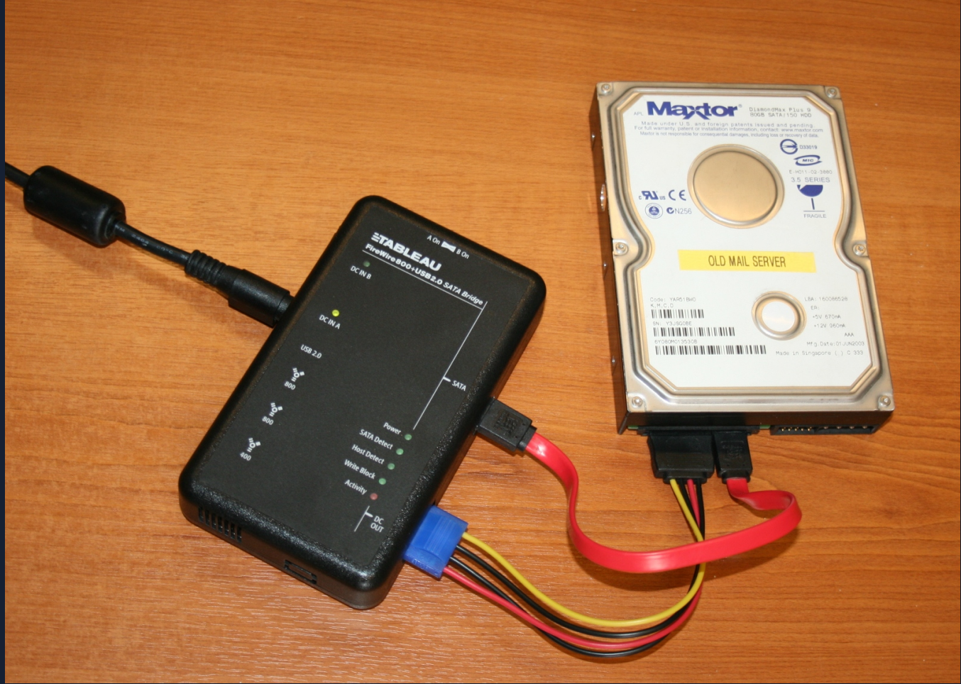
A portable Tableau write-blocker attached to a hard drive (from Wikipedia)
