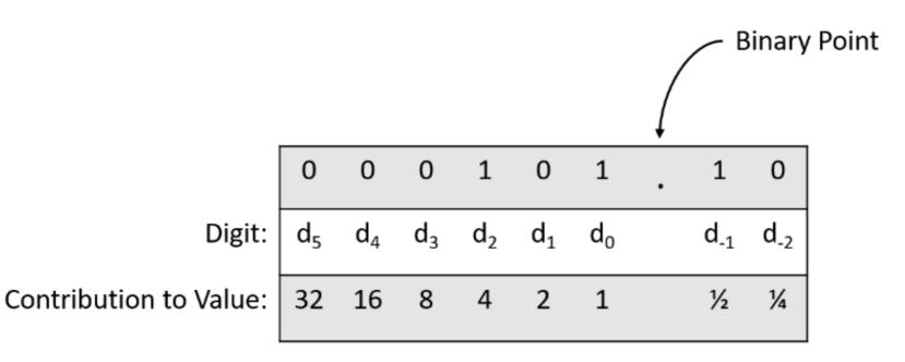
Figure 1. The value of each digit in an eight-bit number with two bits after the fixed binary point
